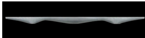
Figure 2.18: Concrete beam made with fabric formwork
